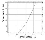
The huge deviation of the forward current will result excess heat that may significantly reduce the LED's lifespan.
