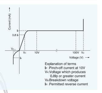
stabilization and current limiting, and perfectly suitable for low current requirements, like a small LED till 18mA.
